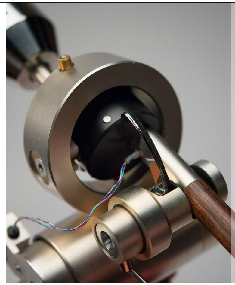
The horizontal bearing also creates a center of gravity offset from the main pivot, which will improve stability and balance. By turning the counterweight assembly, you can adjust the "leaning force" which essentially changes the horizontal damping of the tonearm. Too much damping causes the sound to become muddy and lifeless, while too little makes the sound thin and nervous.
