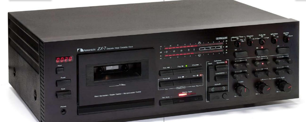
Featuring a discrete three-head design, you could monitor your recordings right from the tape just like an open-reel deck, and the ZX-7 also featured the industry standard Dolby B and the newer Dolby C noise reduction. While Dolby C offered an additional 6 dB higher level of noise reduction than Dolby B, it was more susceptible to problems with head alignment and caused serious "fluttering" in the playback if not perfectly aligned.
