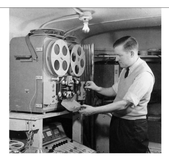
The Mercury recording team employed revolutionary three channel recording techniques and used 35mm magnetic film made specifically for audio recording.
