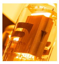
The four output tubes are biased separately, via a very cool little red circular meter on the front of the amplifier. Once the amplifier has been on for a while, with no signal present, adjust the four individual front pots with a plastic screwdriver to 40ma, and you are good to go. During the two months of test listening, the bias did not change a bit or require any adjustment, but I advise checking tube bias every now and then just to be safe. (continued)
