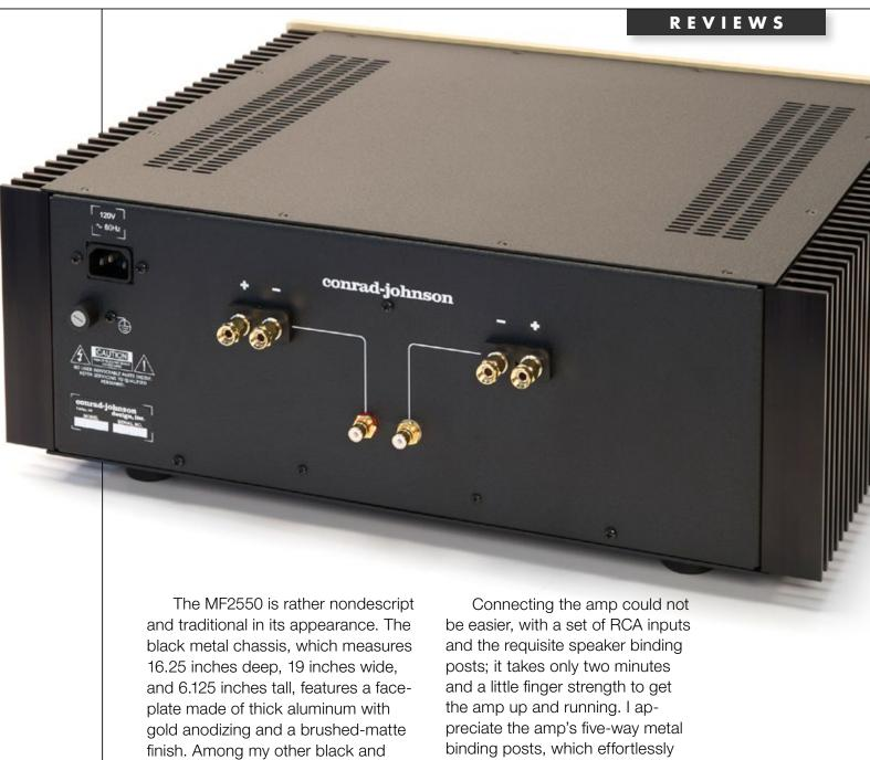
silver audio components, the amp's gold color—a signature of CJ—certainly stands out. The only feature interrupting the smooth faceplate is a power button the size of a quarter on the lower right corner. A gentle yellow LED halo illuminates the button when pressed. The only thing distinguishing the special-edition amp from the standard version is a small plate on the back of the unit that notes the serial number and the SE designation.
