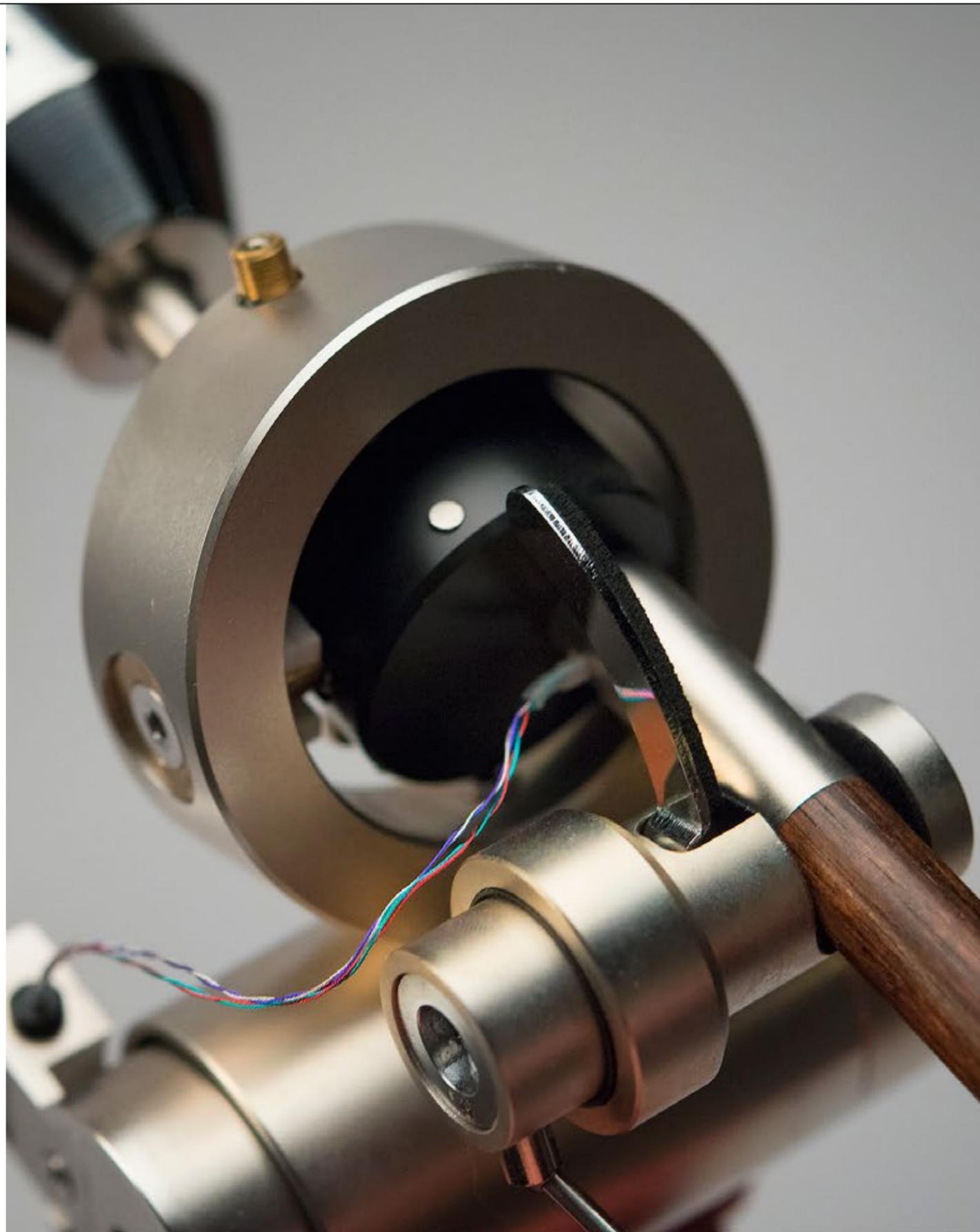
The horizontal bearing also creates a center of gravity offset from the main pivot, which will improve stability and balance. By turning the counterweight assembly, you can adjust the "leaning force" which essentially changes the horizontal damping of the tonearm. Too much damping causes the sound to become muddy and lifeless, while too little makes the sound thin and nervous.
