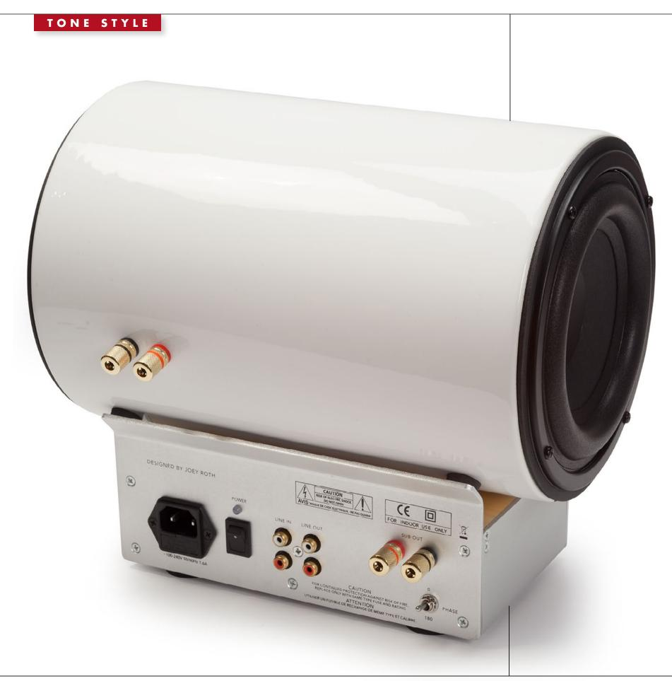
The matching cylindrical subwoofer features a 6.5-inch woofer and passive radiator, with the RCA input jacks set near the active driver. The 40-Hz-rated woofer sits on the curved top of a 50-watt amplifier/crossover. The aluminum-milled casing's front panel is simple, with only knobs for volume control and crossover setting, which is adjustable from 40 Hz to 200 Hz. The back panel holds the subwoofer output, in/out jacks for the source, power-toggle switch, and socket for the two-way power cord.
