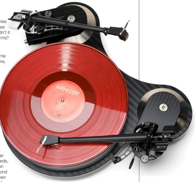
The arm pods screw down with a 5mm hex bolt and can swivel, making it very easy to adjust the pivot to spindle distance of your tonearm. I used the Acoustic Sounds protractor for every arm I worked with and this made removing one arm and resetting another a snap. If you do not have a system that you enjoy, I highly suggest the Acoustic Sounds protractor.
